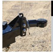
The ultimate in versatility, the 10TV is equipped with an adjustable coupler. This makes it easy to adjust to different hitch heights within a fleet of trucks or to change out to other coupler options.
