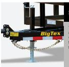
The 8,000# Set-Back Jack allows the tailgate of the tow vehicle to be lowered without the top of the jack damaging the tailgate.
