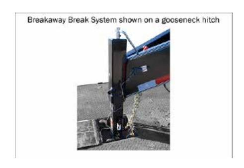
The breakaway brake system may be fitted with a charging facility that draws power from the tow vehicle. If the electrical system on your tow vehicle does not provide power to the breakaway brake battery you must periodically charge the battery on the trailer to keep the breakaway brake system in working order.
