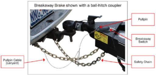
Connect the pullpin lanyard to the tow vehicle so that the pullpin will be pulled out before all of the slack in the safety chains is taken up (see Breakaway Brake System figure). Do not connect the pullpin cable to a safety chain or to the hitch ball or hitch ball assembly. This would keep the breakaway brake system from operating when it is needed.
