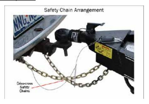
Visually inspect the safety chains and hooks for wear or damage. Replace worn or damaged safety chains and hooks before towing.
